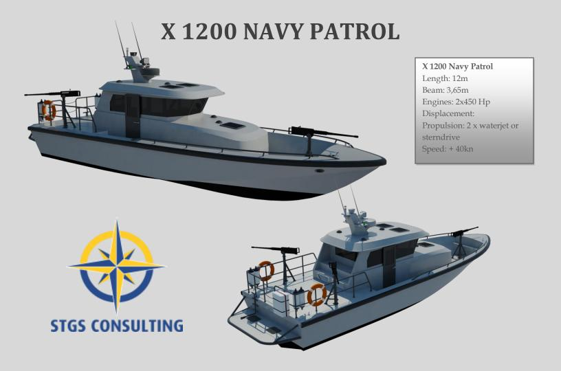
The X 1200 is a multi-purpose platform constructed for an efficient series production as well as for one – off production, extensible in length and width together with a variety of superstructures to meet many kinds of custom fitted configurations. Here as a Search and rescue model, all models are made of marine grade aluminum. High speed crafts combined with waterjet gives outstanding maneuverability and shallow draft capability.
